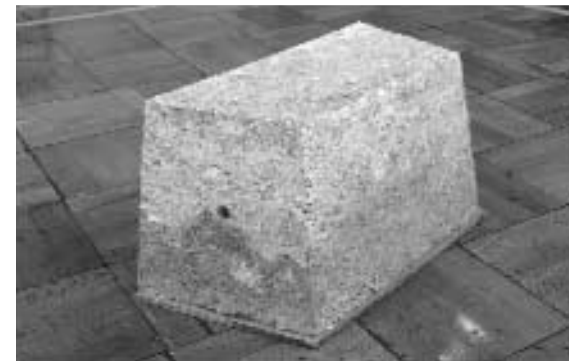
[Paper Brick]: Constructed of rice glue and collected shredded paper.
