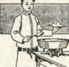
The Box is Fitted for a Small Battery Motor and Heated Water to Heat the Hot Plate.
